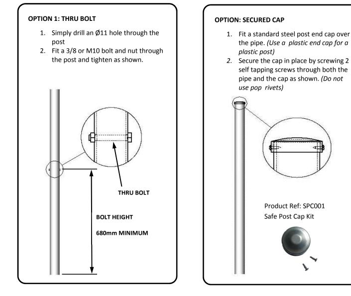
NOTE: Safe -Posts are recommended as Spring Return Signpost Base Units use a spring compressed under high force. In the unlikely event the cable mechanism is released or severed unexpectedly, a Safe Post is designed to arrest the energy of the suddenly released spring, preventing any chance of injury.
